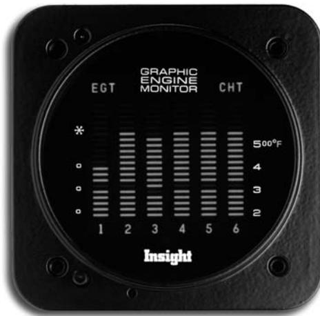
**5. GEM shows:** abnormally low EGT in one cylinder. (Two or more bars lower than the normal indication for your engine).
