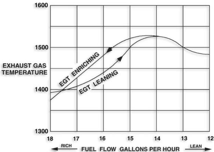
Figure 4. EGT/Fuel Flow for Turbos
