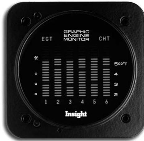
**3. GEM shows:** high CHT readings on one side of the engine (cylinders 1, 3 and 5, or 2, 4 and 6).
