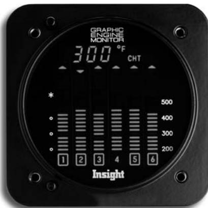
**13. GEM shows:** a drop in EGT for all cylinders in carbureted engines.
