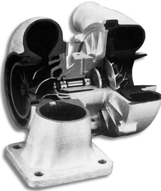
Figure 3. Cut-away view of compressor and turbine
