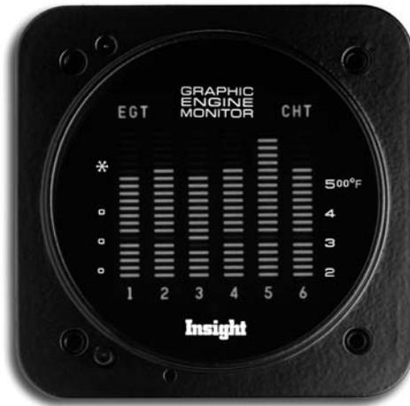
**1. GEM shows:** a gradual or sudden rise in EGT of one cylinder. When temperatures are 50°F above normal the display will blink to warn you of the rise in temperature.
