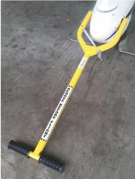
To remove the tow bar, reverse the process, again being careful not to scratch the nose wheel pant as you remove the tow bar.
