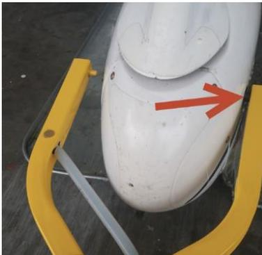
2. Using the crank, tighten the tow bar while keeping it lined up with the passenger-side lug on the nose wheel.
