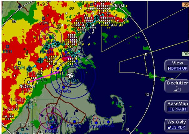
Figure 10.7 Broadcast Datalink Weather
