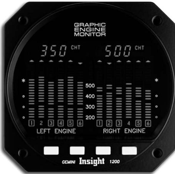
**10. GEMINI shows:** Left engine normal, right engine has a slight drop in EGT and rising CHT indications in one or more cylinders possibly accompanied by engine roughness.
