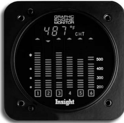
**7. GEM shows:** high CHT on one or more cylinders under all conditions after engine overhaul.
