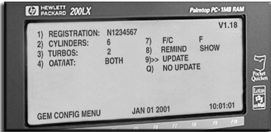
Characteristics of the GEM 610 and the GEMINI 1200 Displays are controlled by the GEM CONFIGURATION. The GEM CONFIG function reads and updates the GEMs configuration status.
