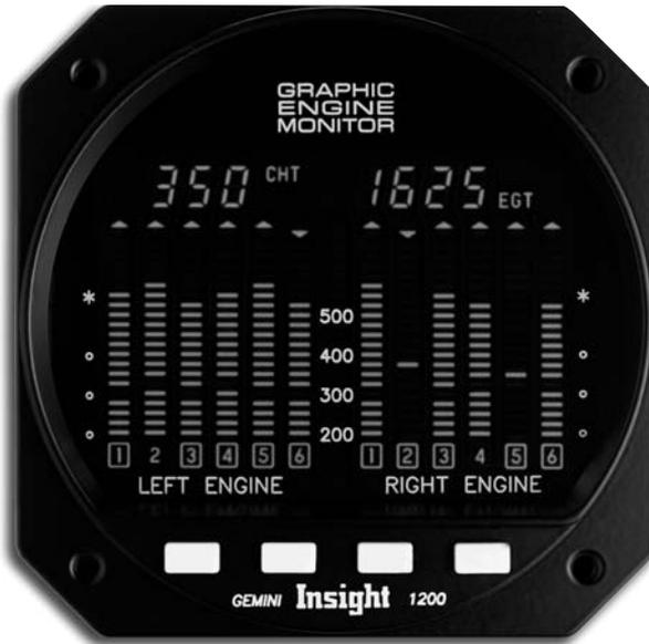
**14. GEMINI shows:** Black CHT bar missing in one or more columns on the left engine, entire EGT columns missing on the right (CHT bar automatically reverses color to remain visible).
