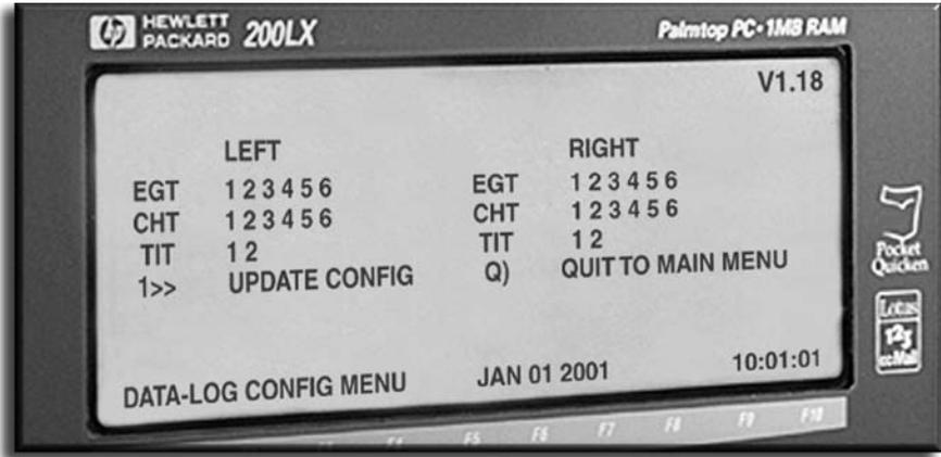
The DATA-LOG CONFIG controls which temperatures are recorded during the data-log process. The DATA-LOG CONFIG will by default mirror the GEM CONFIGURATION but can be modified by turning-off unwanted channels.
